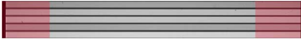
Fig. 27 Non-uniformity matrix of the 5 visible filters (415 nm band to 690 nm band, top to bottom). The red shading is not part of the system response but rather delimits portions of the CCD readout in multispectral mode. Monochrome images are acquired with the 645 nm filter (4th band from top)
