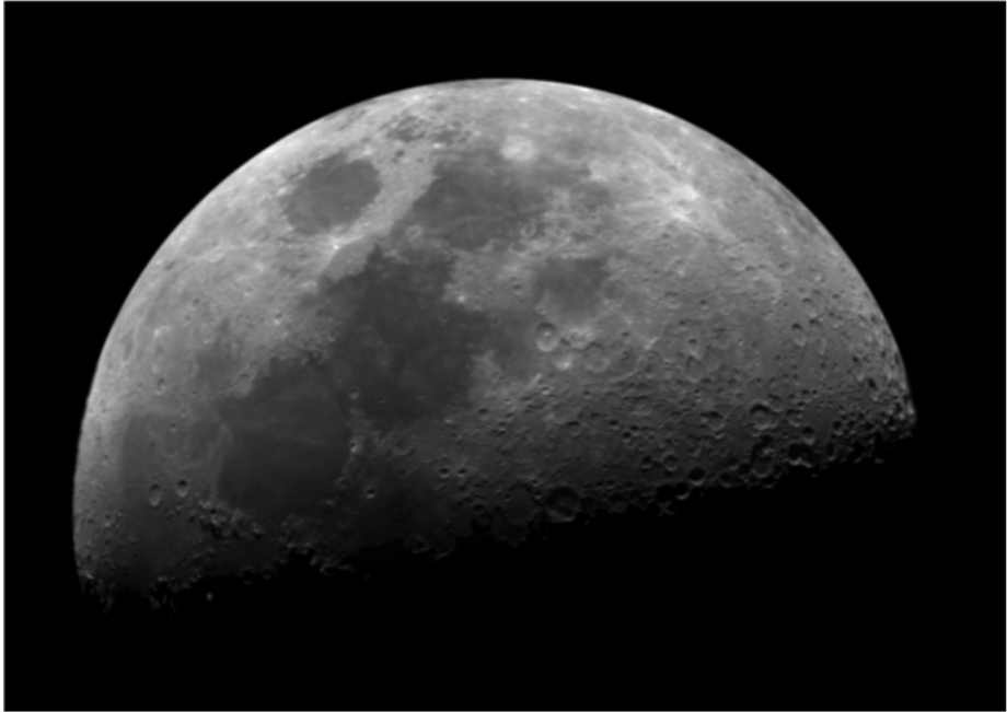
Fig. 21 NAC-L image of the Moon obtained immediately after removing instrument from thermal vacuum testing. Slight deviations from sphericity are due to scanning the NAC by hand, Moon is about 940 pixels in diameter
