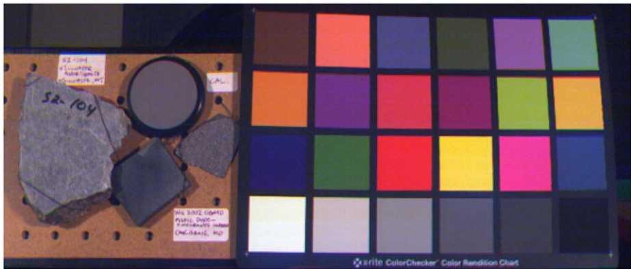
Fig. 30 WAC RGB composite (RGB: 689, 643, 415 nm) of standard Munsell Color chart and geologic samples
