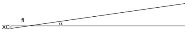
Fig. 16 Idealized camera geometry. Here xc/fl = \tan(\alpha) , where xc is the mm coordinate of the undistorted image, and fl is focal length in mm, and \alpha is the angle from the optical center
