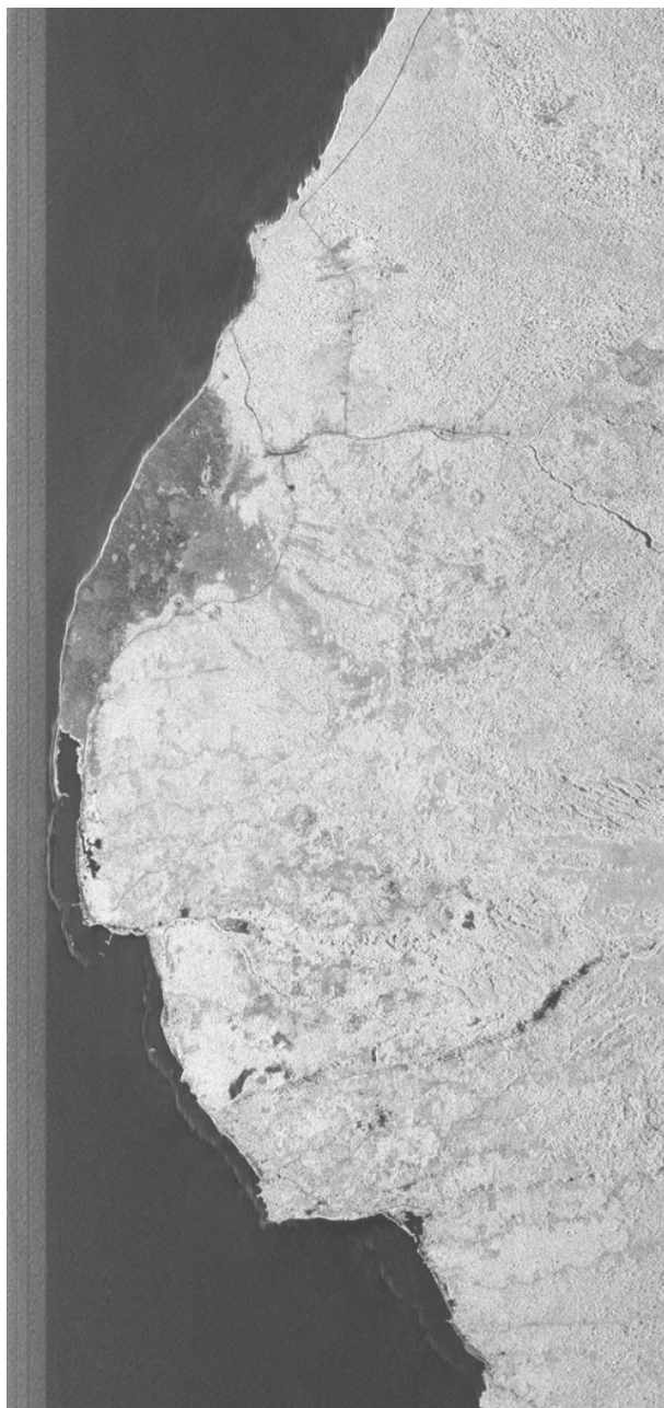
Figure 25: Example (Savaii293-1) where the cross-talk removal algorithm has obtained an incorrect result for the HV-pol scene in the near range due to low signal-to-noise. The failure is highlighted by the bright near-range (left side) streaking. The implication is that all of the signal over the ocean in the near range for the cross-pol channel is cross-talk noise. The cross-pol terms in the scattering matrix here are below the AIRSAR noise threshold.
