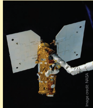
[Above] Launched from the Space Shuttle Challenger in October 1984, the Earth Radiation Budget Satellite was designed to investigate how energy from the sun is absorbed and re-radiated by the planet, also known as the energy budget.
