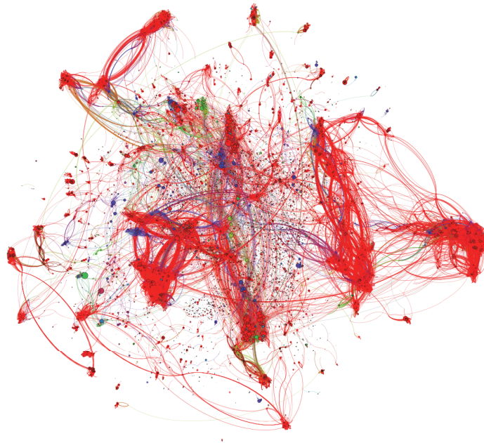
Fig. 1. The landscape of solutions for “gradient descent for linear regression” representing over 40,000 student code submissions with edges drawn between syntactically similar submissions and colors corresponding to performance on a battery of unit tests (red submissions passed all unit tests).
