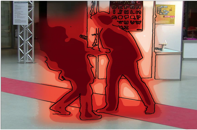
Figure 2: The silhouettes of two people fighting. The red color indicates that an anomalous event is happening.
