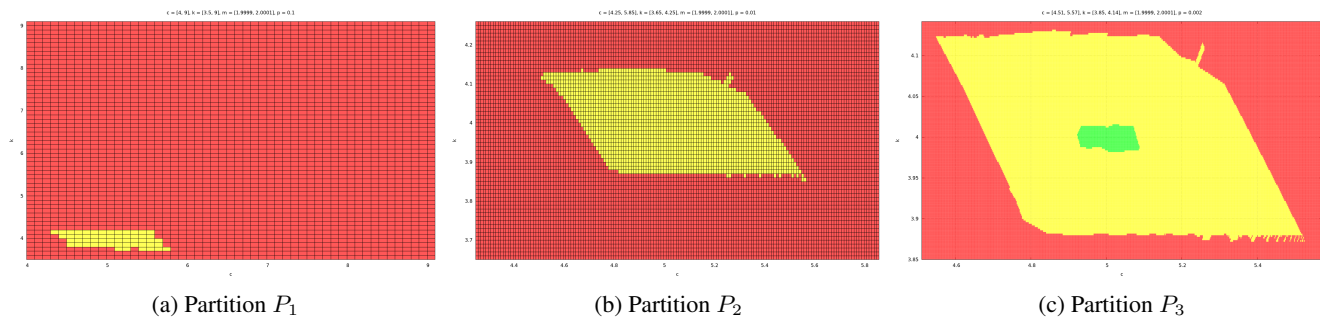
Figure 11 – Partitions and estimation results (red, yellow and green boxes are resp. rejected, undetermined, accepted parameters values).
