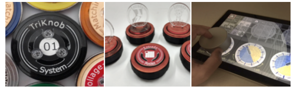
Figure 1. Fabricated and commercially available tangibles. Laser cut knob (left); 3D printed knob (center); Surface Surface Dial (right).
