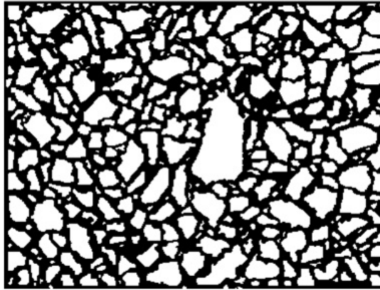
Figure 4. Formation of ore particle images using the "watershed" algorithm
