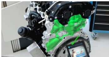
Figure 2: Superimposed 3D data of an engine part visualized using a head-mounted display.
