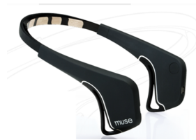
Fig. 1. The MUSE device used for acquisition of the EEG [24].
