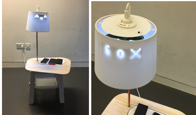
Figure 6. Lamb Lamp brightens up and smiles when all smartphones are together; it pops up a random number indexing a game set under the table.
