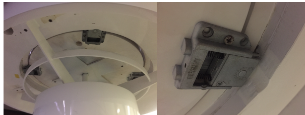
Figure 4. Rotating track of the outer ring inside Swing Compass Table
