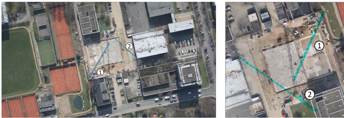
Figure 12: Orthorectification and georeferencing of labels: aerial image with labeled tower crane (left); orthorectified and georeferenced labels stored as GeoTIFF (right)
