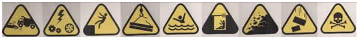
Figure 1: Pictograms of nine critical risks in hydroelectric powerhouses
