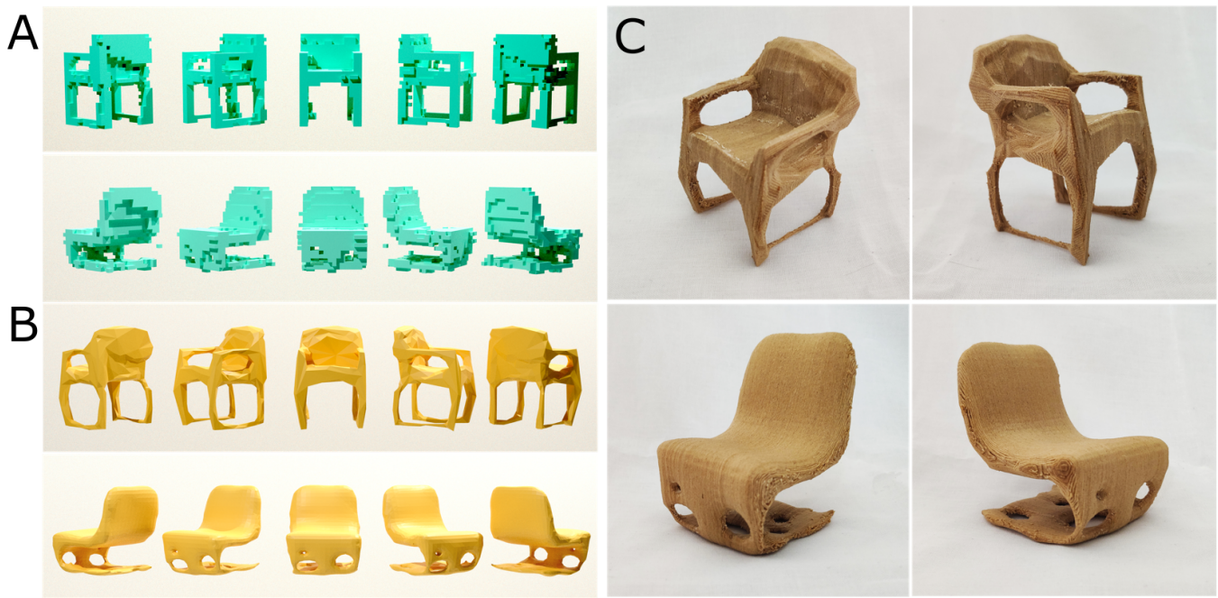
Fig. 3: Results Main results of the VAE at different stages. A.) First outcome of the network expressed in voxels with a 32 \times 32 \times 32 resolution. The figure shows the values of two different outputs from the same class (chairs). B.) Shows the results shown in A after smoothing. C.) Shows the outcome of our VAE in real scenario. The results obtained from the algorithm are now obtained through additive manufacturing.
