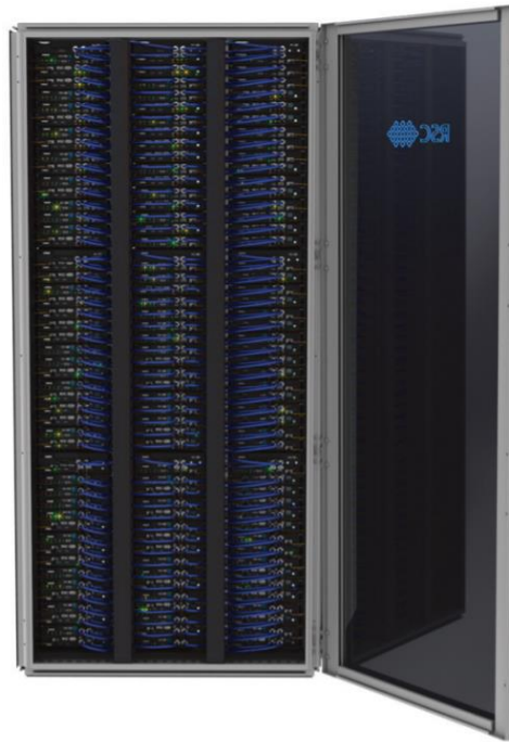
Fig. 3. RSC hyperconverged platform for HPC
