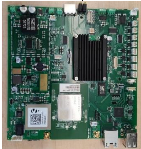
Figure 16: Power distribution and Spoofing detector PCB board
