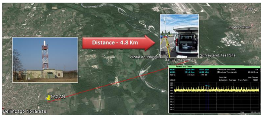
Figure 19: Example of a Live RFI source scenario over E5a/L5 band
