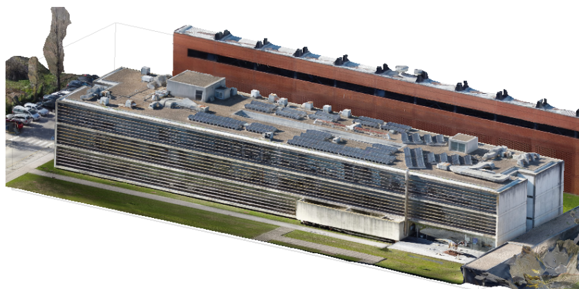
Figure 7: Point cloud in building texture – SE façade in Metashape
