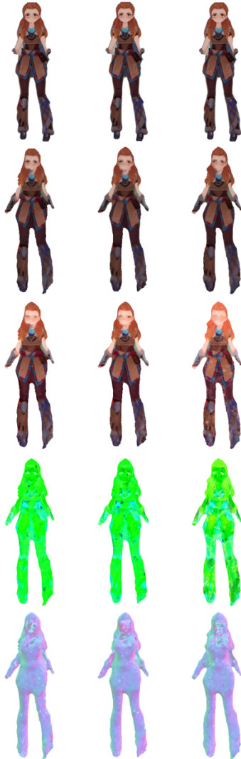
Figure 8: Validation results over the first sample for different center estimations on the game character. Left to right, GRASP, BB, and averaged. Top to bottom, ground truth, rendered reconstruction, diffuse texture, specular texture, and normal map. Images have been cropped for visibility.
