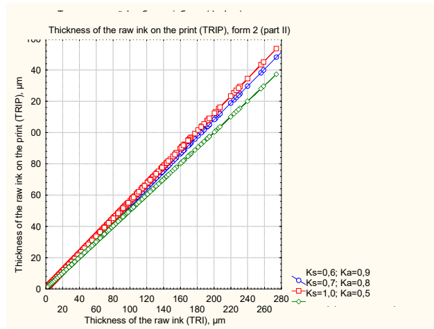
Figure 13: The regression dependence of the thickness of the raw ink on the p rint from the thickness of the raw ink (the stencil form with a copying layer that exceeds the grid thickness by 100 μm), if the coefficients of spreading and absorption are located in opposite directions
