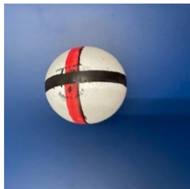
Figure 5: Photograph of table tennis ball with black and red lines as marker
