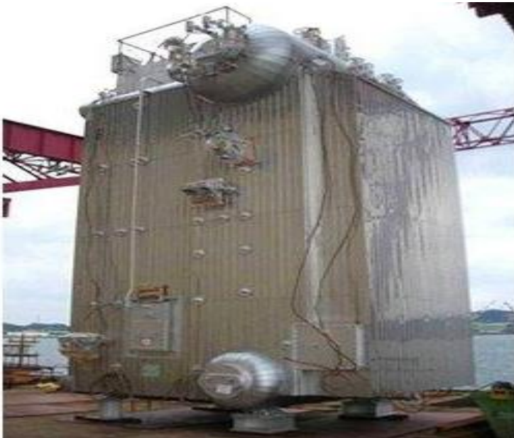
Figure 3: Photograph of a Mitsubishi MAC 35 marine steam boiler [6]
