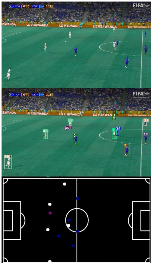
Figure 9: The result of combining the player finding model and the homography matrix definition model
