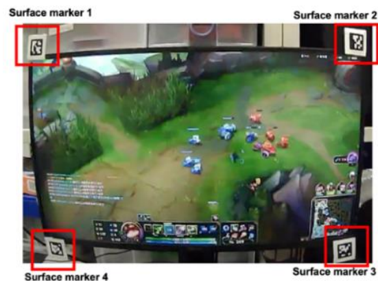
Figure 1: Surface markers and experimental environment. Each red box indicates the surface marker used for detecting the monitor screen and calibrating the gaze movement.
