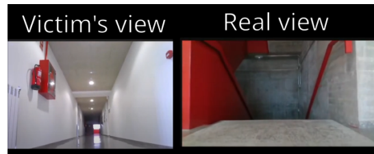
Figure 3: On the left, view of the teleoperator after being attacked. On the right, real image of the robot's situation.
