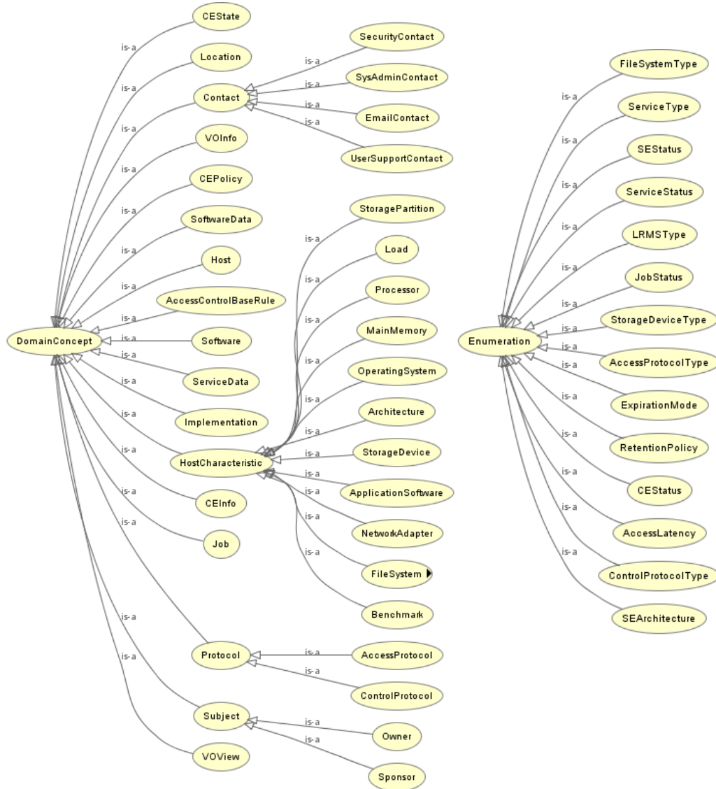
Fig. 2 shows the class hierarchy of DomainConcept and Enumeration classes, which are used to describe the basic elements the Grid system.
