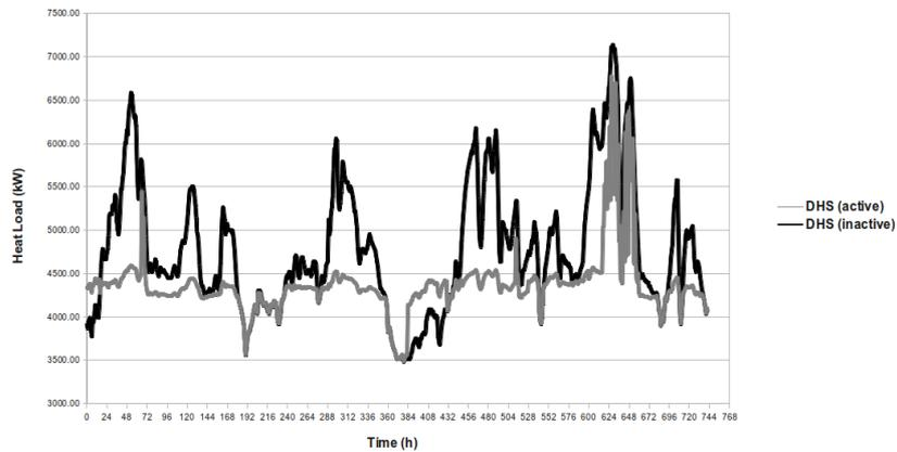
**Fig. 4.** Comparison between active and inactive distributed heat storage
