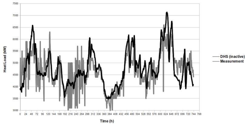
**Fig. 3.** Comparison between DHEMOS and measured data
