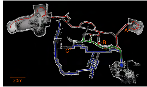
Fig. 13. Result from DARPA Subterranean Challenge Final Competition in Louisville Mega Cavern, KY. Three vehicles with red, green, and blue trajectories are deployed running TARE and FAR planners together. The segments between A and B on the red trajectory and between the start point (blue dot) and C on the blue trajectory use FAR planner to transit. Other segments on the trajectories use TARE planner to explore.
