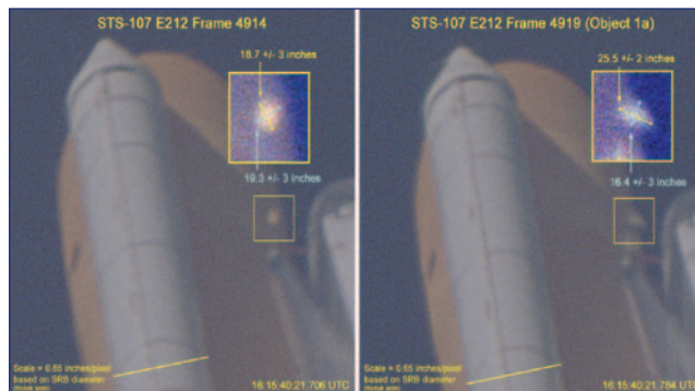
Figure 3-6. Photographic analysis techniques determined foam size: debris appears almost circular in frame 4914 and elongated in frame 4919.
