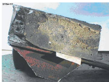
Figure 9.7. Tile Item 57754 bonded to section of carrier panel
