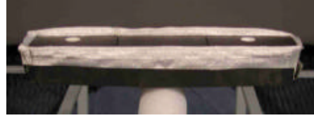
Carrier Panel Segment with Horse Collar
