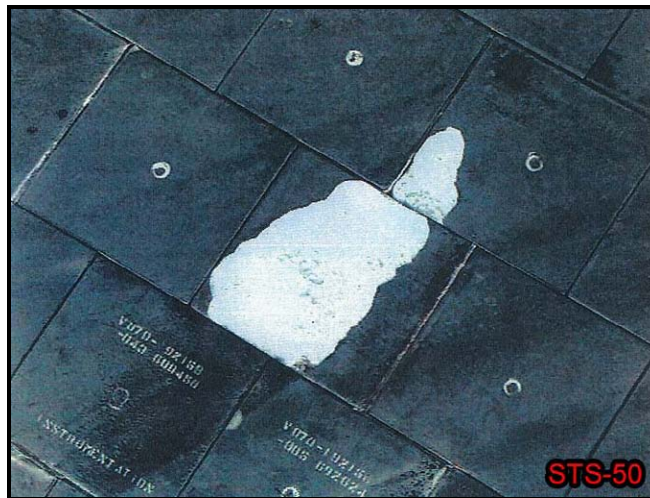
Figure 4.4.5.2b Detailed view of wing tile damage, STS-50
