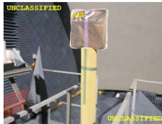
Figure 9 –Thermal Blanket on Low RCS Support at the AFRL Compact Range.
