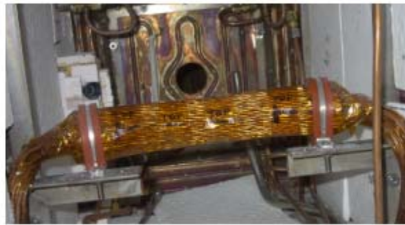
Figure 6-36: Wire bundle arc jet testing (before test)
