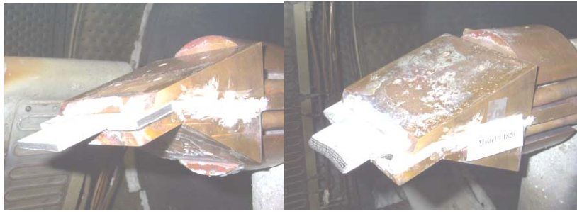
Figure 6-93 -Test #3 Pre and Post Test - Knife-Edging Apparent
