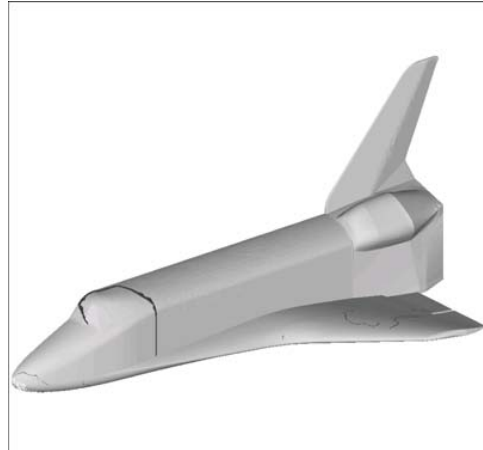
Figure 4.7-18a&b Baseline Clean Geometry (a) – no Vertical Tail & (b) with Vertical Tail
