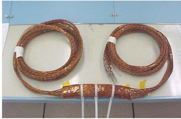
Figure 6-27 – Cable Bundle Test Article
