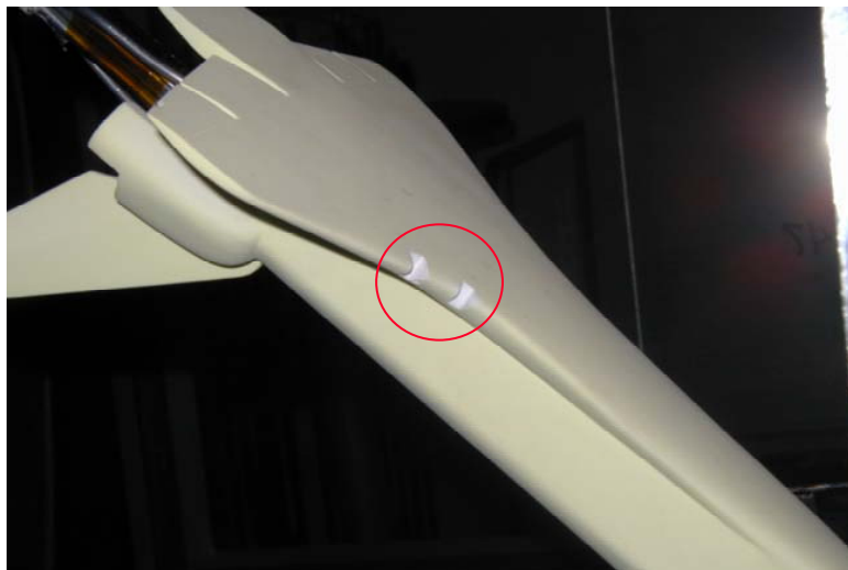
Figure 4.1-6 WT Model with WLE RCC panels (6 & 9) removed
