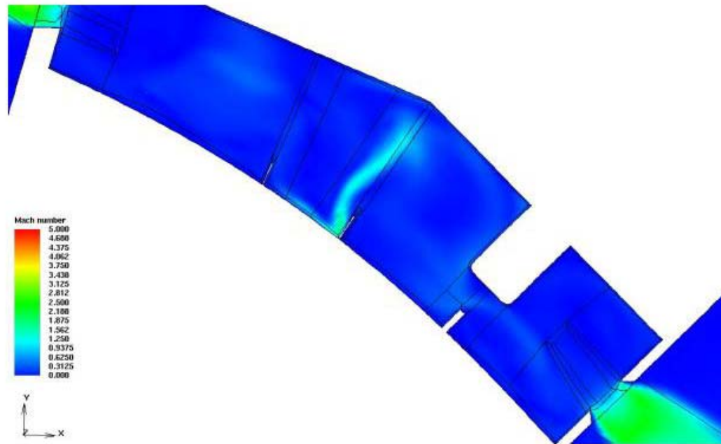
Figure 5.3.6-23 Mach Contours from Panel 7 Hole Coupled External/Internal Flow Simulation I (Z=301.6; Postprocessed using every other point)
