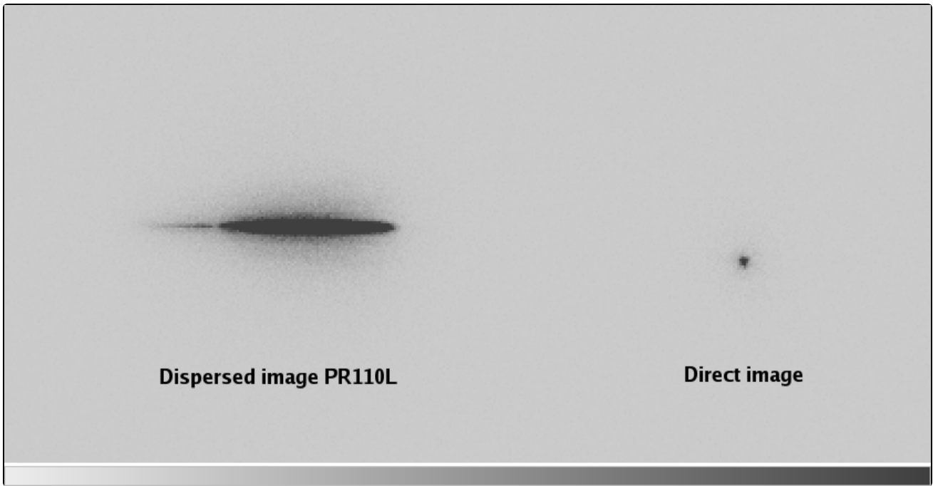
Figure 6.23: Sum of direct (F122M) and PR110L prism exposure of the standard star WD1657+343.
