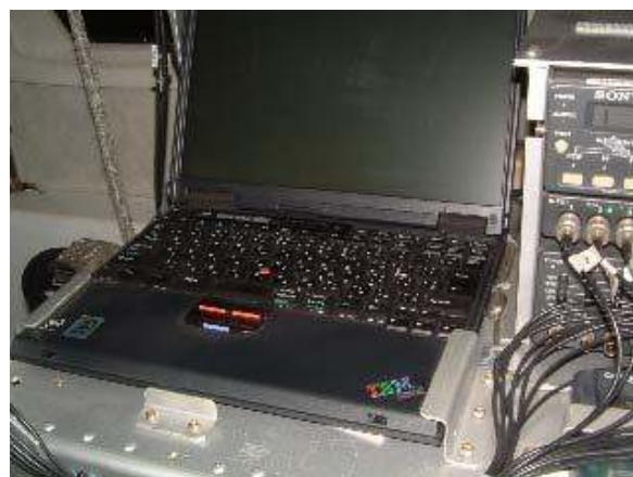
Figure 7.42 Computer secured with metal brackets
