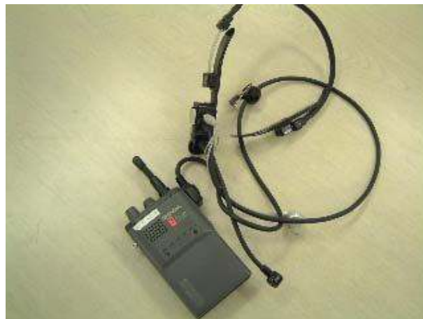
Figure 7.68 Intercom (Two-minute warning and now signals - at entry into microgravity - during flight over an intercom from the pilot)
