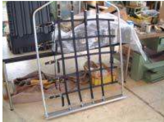
Figure 7.70 Flexible net between the pilot cabin and passenger area (Prevention of floating experiment equipment or samples from reaching the pilot during the flight)
