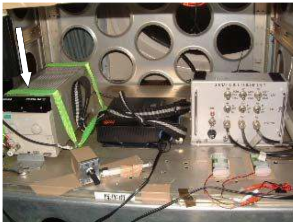
Figure 7.29 Experiment equipment secured with DAS-specified belts
