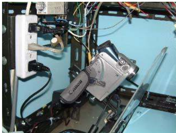
Figure 7.48 Camera firmly secured to counter the Influence of microgravity
