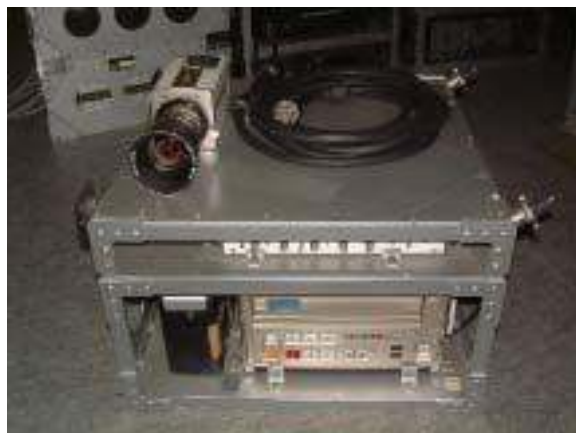
Figure 7.51 High-velocity camera (mount recorder on rack as well)
