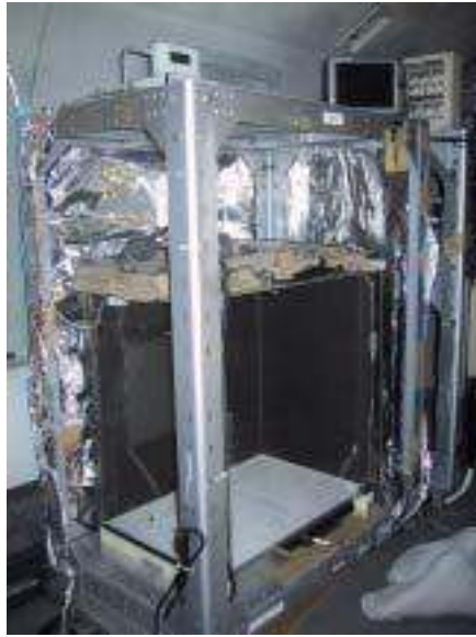
Figure 7.36 Aluminum foil around your components to block noise
