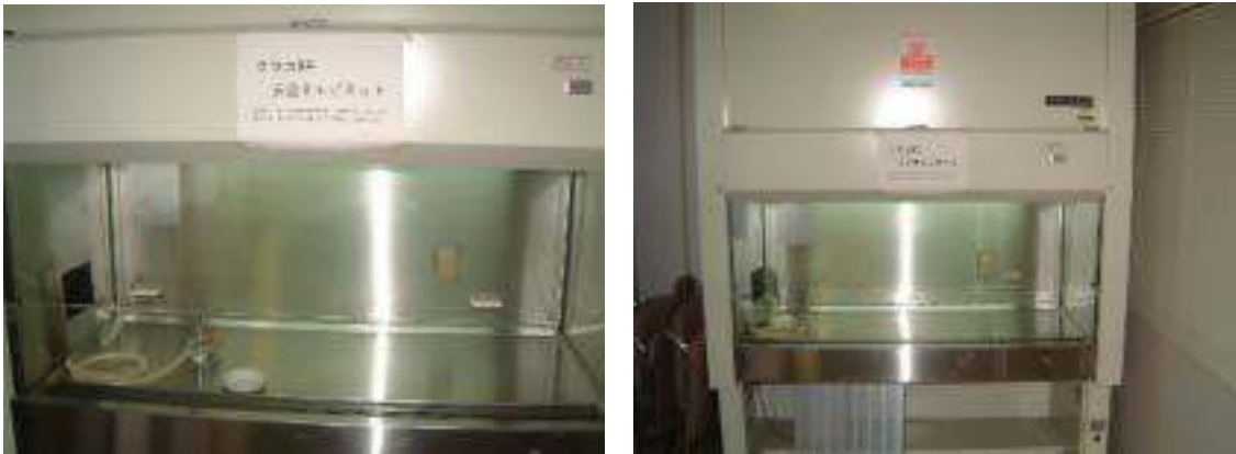
Figure 7.22-1 Experiment equipment inside the preparation room for life-science experiments: Safety cabinet
