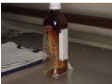
Figure 2.7 Water creeping up the wall of the plastic bottle under microgravity
