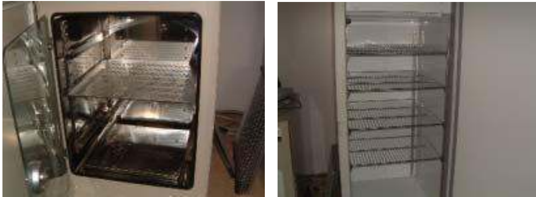
Figure 7.22-3 Experiment equipment inside the preparation room for life-science experiments: CO2 incubator(left) and Research refrigerator(right)
