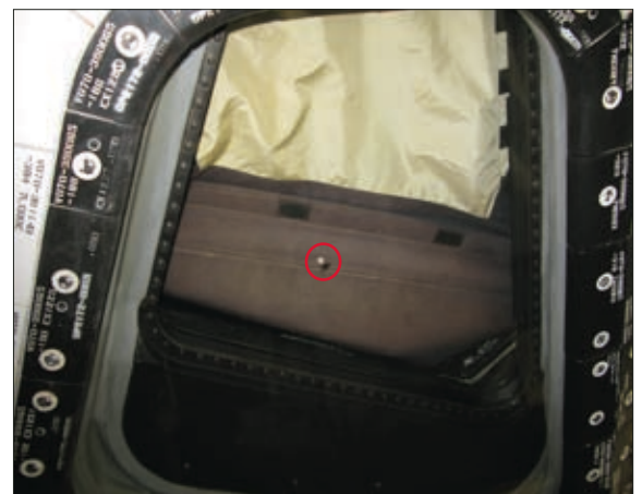
Figure 2. STS-126/OV-105 window #6 impact damage location.
