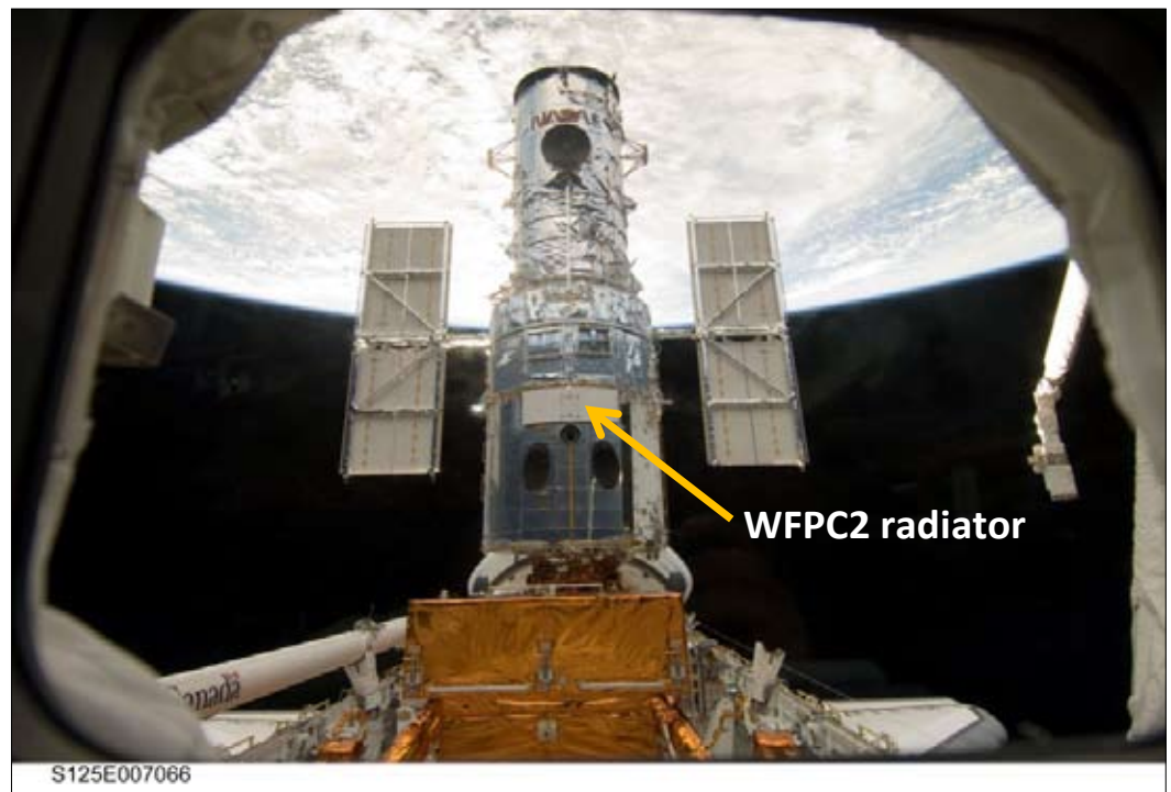
Figure 1. A view of the HST after it was captured and locked to the Atlantis cargo bay during the 2009 servicing mission. (NASA Photo/s125e007066)
