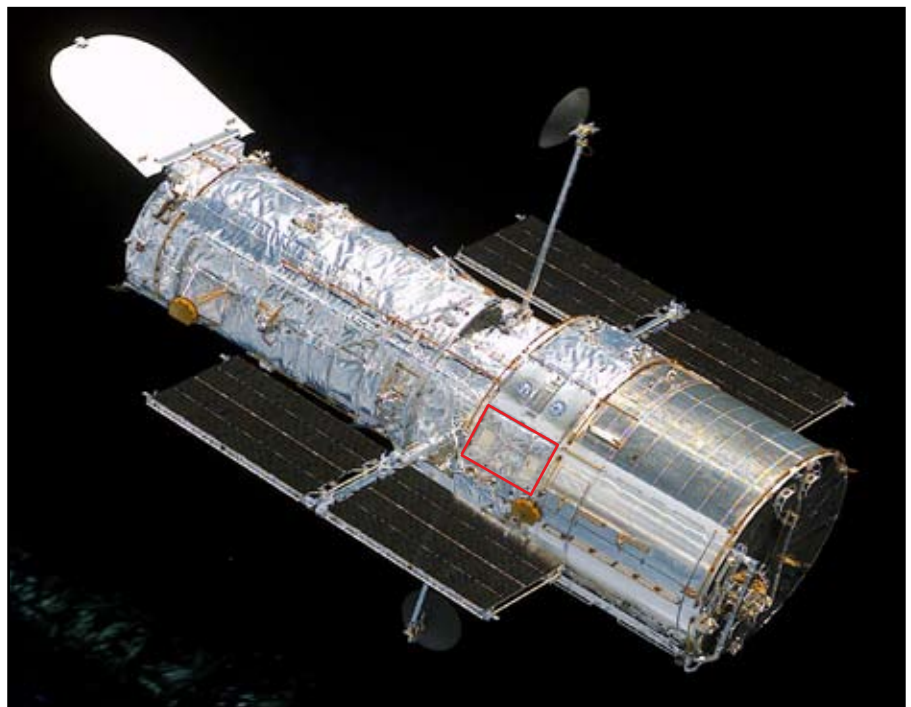
Figure 1. An image of the Hubble Space Telescope. The Bay 5 MLI is outlined by red lines. (edited NASA Photo/S109E5700)
