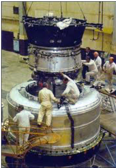
Figure 1. Briz-M central tank and main engine being inserted into the APT.
