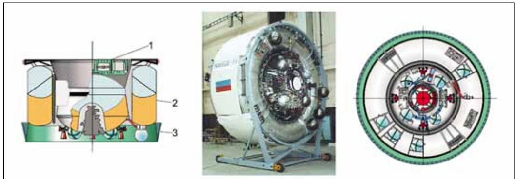
Figure 1. The Briz-M upper stage contains a central engine and propellant surrounded by an auxiliary propellant tank, which is ejected part-way through the mission.
