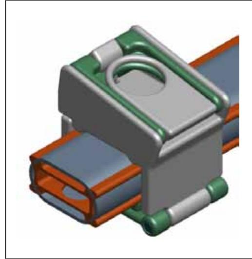
Figure 7. Example of clamp tool to mitigate MMOD damage to handrails.
