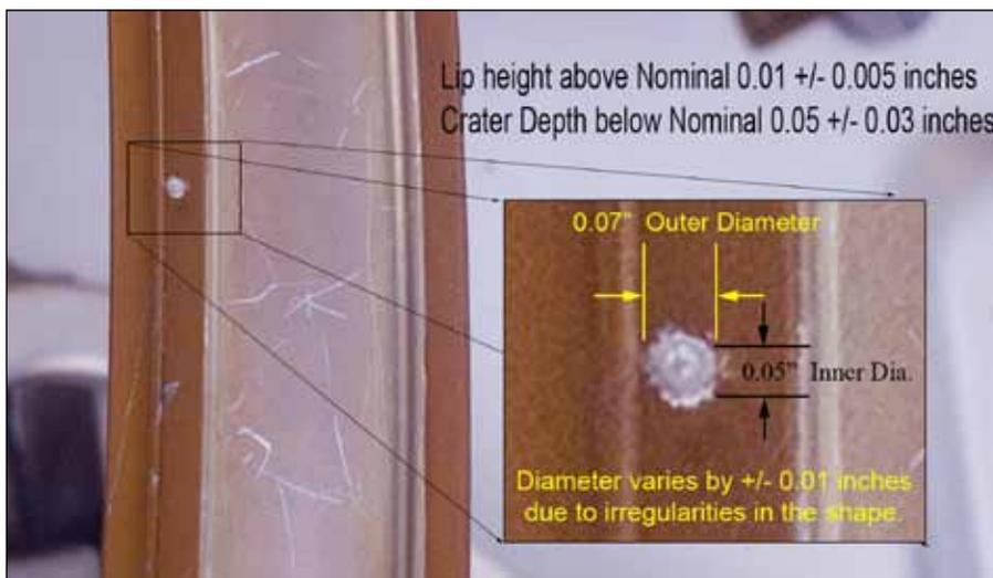
Figure 5. Crater on airlock handrail photographed during an STS-122 EVA measures 1.8 mm (0.07 inch) outside diameter with 0.25 mm (0.01 inch) crater lip height (JSC Image Science and Analysis Group).
