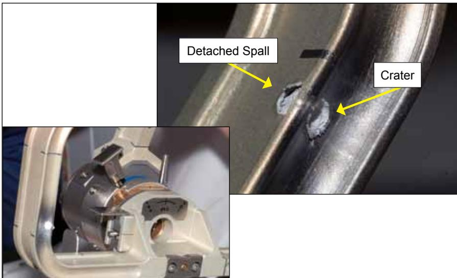
Figure 4. Nearly 5-mm-diameter crater found by ISS crew on the EVA D-handle tool stored externally on ISS, prior to STS-123 EVA. Note that the detached spall from the side opposite the MMOD impact crater also has sharp edges. The D-handle is made from similar materials as typical ISS dog-bone handrails.
