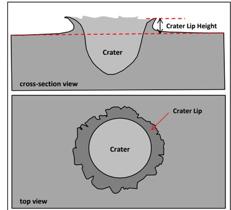
Figure 1. MMOD impact craters in metals typically exhibit raised sharp-edged "crater lips." Top image shows a cross-sectional (side) view of the crater and associated crater lip. Bottom image shows the top view of the crater.
