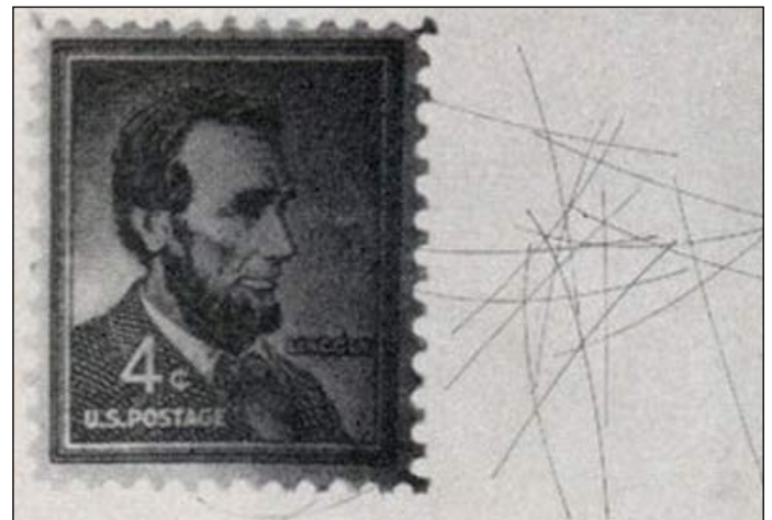
Figure 1. The West Ford Needles were individually small, but in a large group they possessed useful radar reflective qualities. For scale, compare the needle sizes in relation to the postage stamp (enlarged to show detail).
