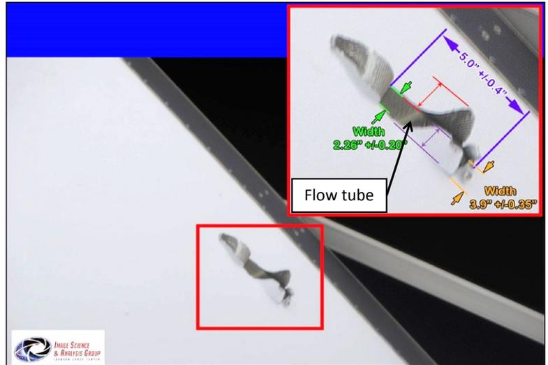
Figure 2. Close-up of exit damage.
