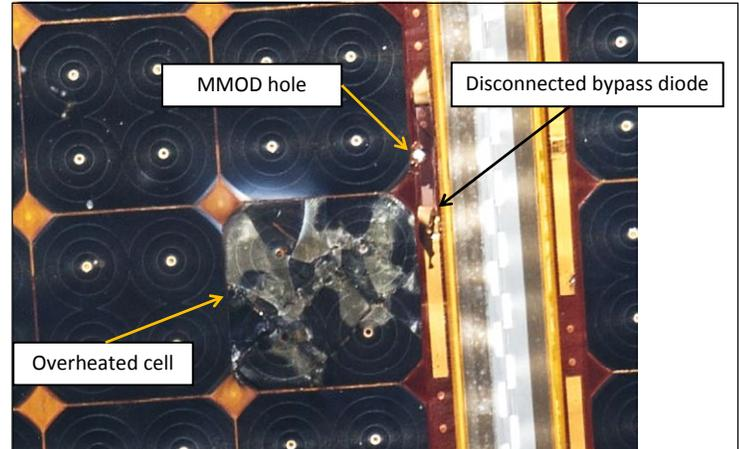
Figure 6. ISS Solar Array 2A, panel 66 damage.
