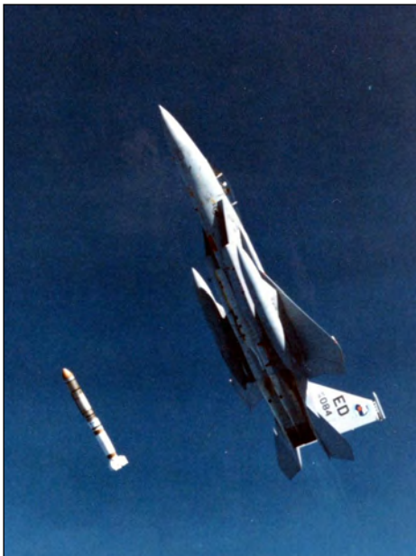
Figure 1. The Boeing F-15A-Eagle, named “Celestial Eagle,” as observed from a chase plane during the ASAT missile launch, 13 September 1985 (U.S. Air Force). The antisatellite missile is shown shortly after separation from the F-15, but before ignition. The missile will release a miniature homing vehicle to destroy the satellite on impact.
