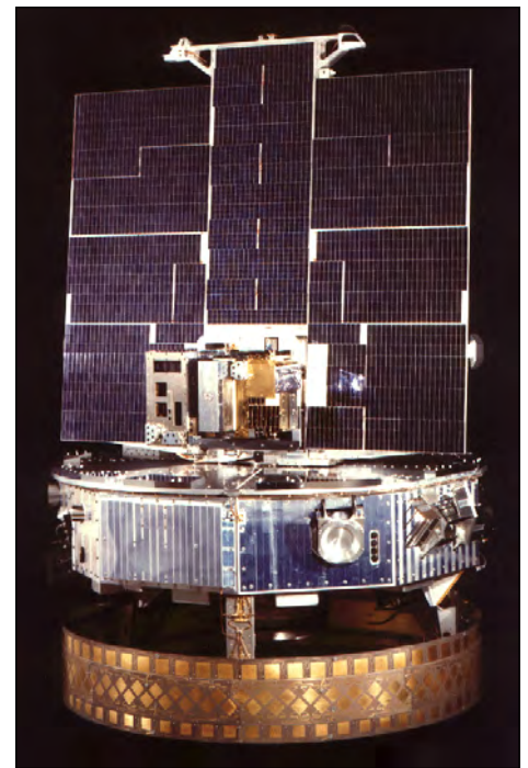
Figure 3. The Space Test Program spacecraft P78 was launched on 24 February 1979 with a mission to obtain scientific data from Earth- and Sun-oriented experiments. Included with its instrumentation was a white-light coronagraph and an ultraviolet imager; the combined package was designated Solwind. The platform was of the Orbiting Solar Observatory type, with a solar-oriented sail and a rotating wheel section. It remained partially operational until it was impacted during the ASAT test. Image courtesy of NASA Goddard Space Flight Center, NASA’s HEASARC: Observatories. Available online at: https://heasarc.gsfc.nasa.gov/docs/heasarc/missions/p78-1.html .
