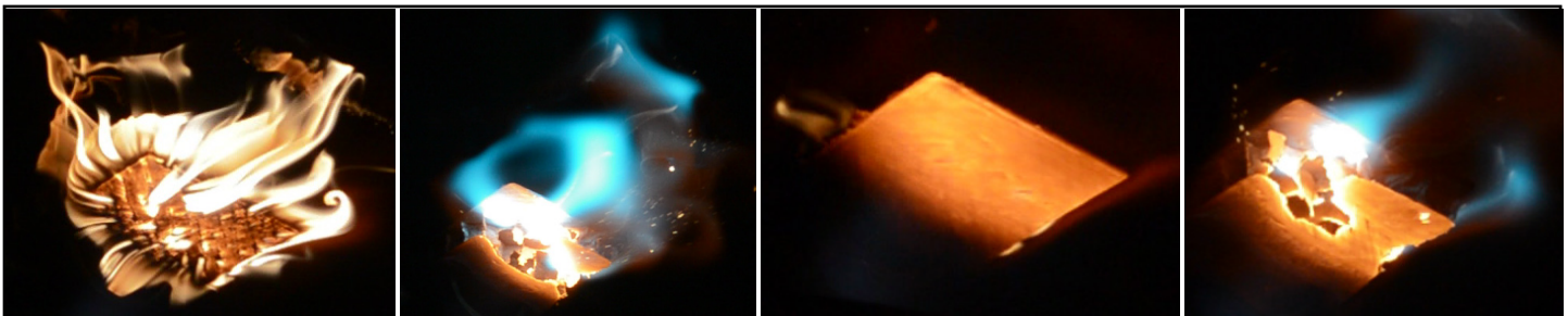
a) Epoxy phase change from solid with volatiles charring and burning.
