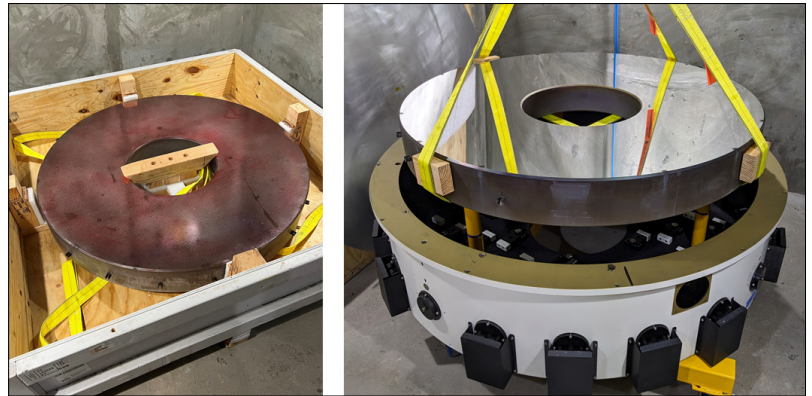
Figure 3. (a) ES-MCAT's primary mirror with the old reflective coating placed in the shipping crate, ready for transport. A layer of First Contact polymer was applied to the mirror for protection. (b) The primary mirror with a new reflective coating being lowered into the primary mirror cell for installation in the telescope.
