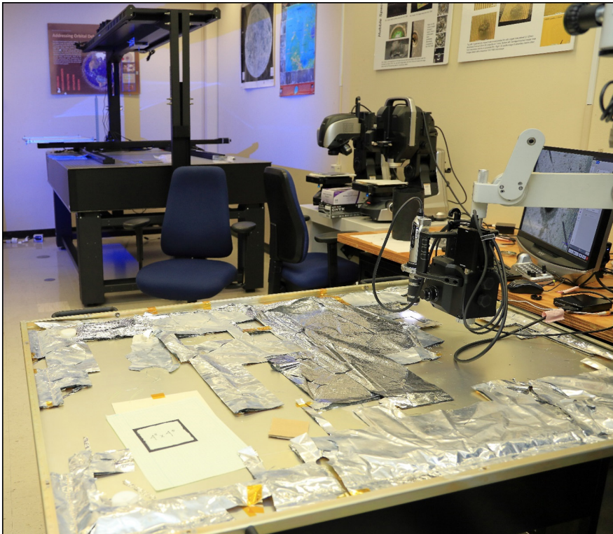
Figure 5. Overview of KEYENCE microscopes in FAF analyzing a multilayer insulation blanket that was returned from HST on STS-125.
