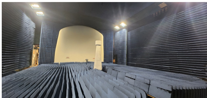
Figure 2. View of the OSU-ESL compact radar range showing the reflector on the back wall and the rotating low density foam positioner in the center. The chamber is lined with RF absorptive wedges designed to minimize reflection of RF waves from the walls.
