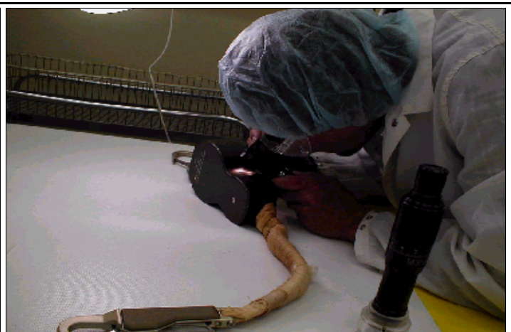
Figure 2. Inspection of 21.2 cm (8.4 in) long tether housing.
