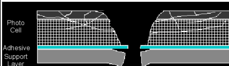
Figure 3. Characteristic Solar Cell Impact Damage (cross-section)
