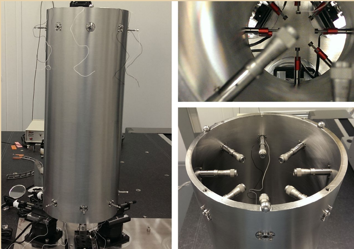
Fig. 5. Left: The completed reaction structure with installed micro and coarse adjusters. The reaction structure sits on three alignment positioning stages used to level it to gravity. Right top: A close-up of the lower, remote coarse adjusters. Right bottom: A close-up of the upper, manually operated coarse adjusters.
