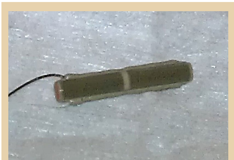
Fig. 1. A Xinetics radial electrostrictive adjuster. The adjuster is ~4 mm in diameter and 25 mm long. Applying voltage via the black and (barely visible) white leads changes the length of the adjuster. Electrostrictive devices maintain their dimensions even when voltage is removed.
