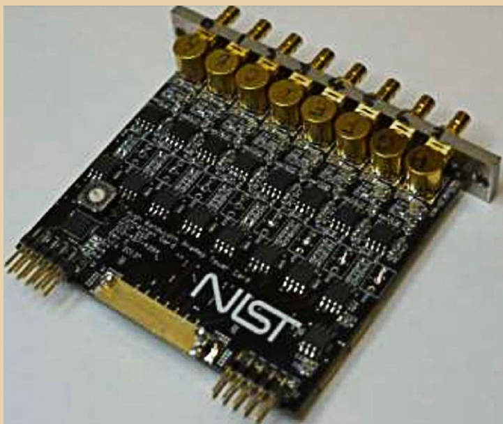
Fig. 3. Room temperature analog amplifier capable of reading out eight columns with high bandwidth.
