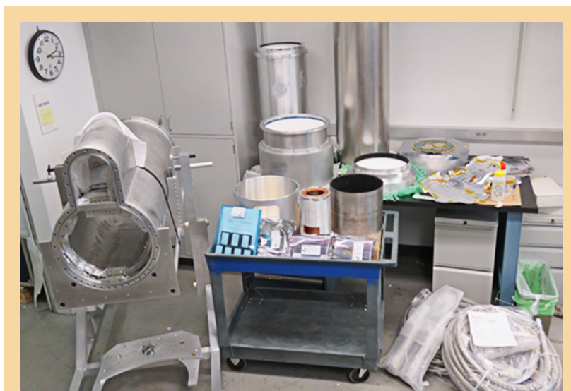
Fig. 7. Test bed for checking RF performance and carrying out future 200-350-GHz antenna development. The system is a small telescope cooled to 4 K using a pulse tube combined with a 300-mK cooler for operating the detectors.
