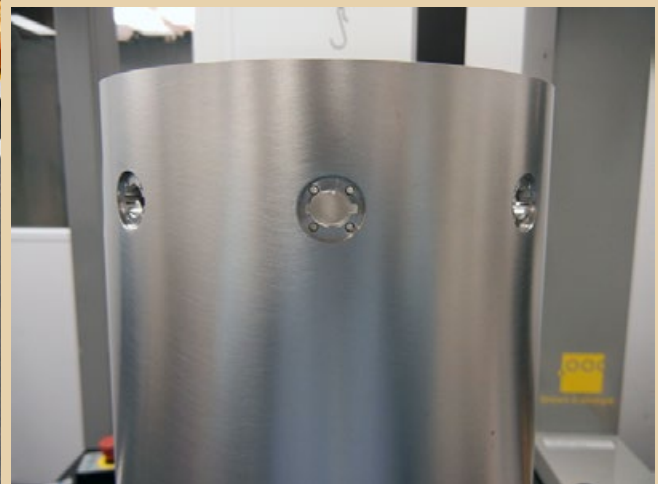
Figure 5: Left – photo of reaction structure for the 23 cm diameter single shell test. The structure is resting on a stage prior to being measured on the SAO CMM. Three mounting points can be seen at each end for six of the 16 adjusters. In the close-up photo, above right, can be seen a detail of the adjuster attachment points.
