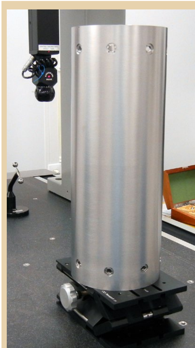
Figure 5: Left – photo of reaction structure for the 23 cm diameter single shell test. The structure is resting on a stage prior to being measured on the SAO CMM. Three mounting points can be seen at each end for six of the 16 adjusters. In the close-up photo, above right, can be seen a detail of the adjuster attachment points.
