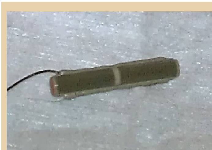
Figure 1: A Xinetics radial electrostrictive adjuster. The adjuster is ~ 4 mm diameter and 25 mm long. Applying a voltage via the black and [barely visible] white leads changes the length of the adjuster. A property of electrostrictive devices is that they maintain their dimensions even when voltage is removed.
