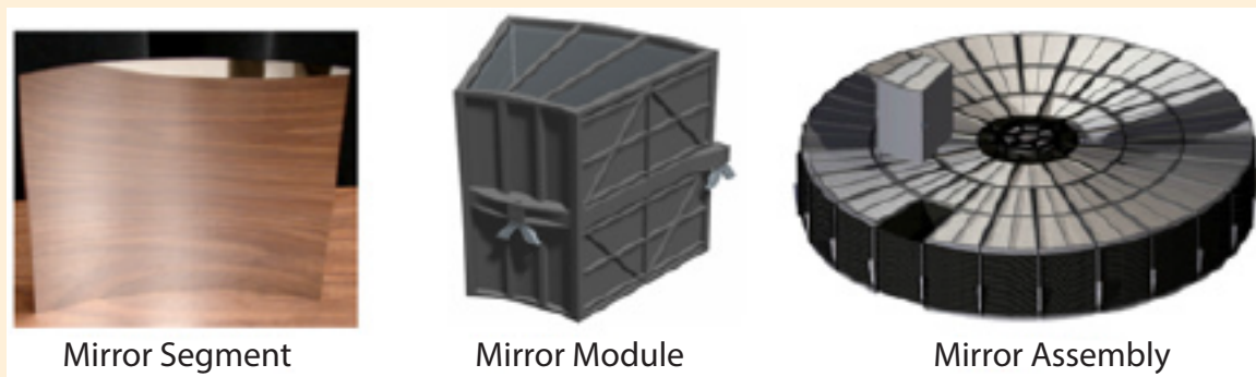
Figure 3.1–1. The hierarchical structure of a segmented design is shown. Left: mirror segment; Center: mirror module, and; Right: telescope mirror assembly. Nominally, a mirror segment is 200 mm × 200 mm; a mirror module contains ≈100 co-aligned mirror pairs (primary and secondary); and a telescope mirror assembly comprises of order 10–100 aligned and integrated modules.
